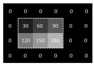
The block or object serializes the image from left to right, one line at a time. The timing diagram shows the control signals and pixel data that correspond to this image. The diagram shows the serial output of the Frame To Pixels block for this frame.
